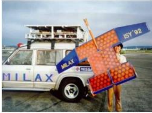
Figure 2.21 Piloting an Airplane Powered by RF Energy (Freq = 2.411 GHz) (Matsumoto, 2002)
