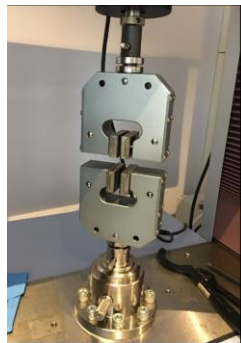
Figure 3.21: UTM device exhibiting tensile specimens mounted with pneumatic tensile jaws.
