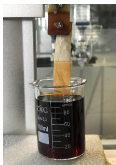
Figure 3.7: a) Coating of randomly oriented PBI nanofibers produced at 15wt% using 50 mM catalysis solution.
