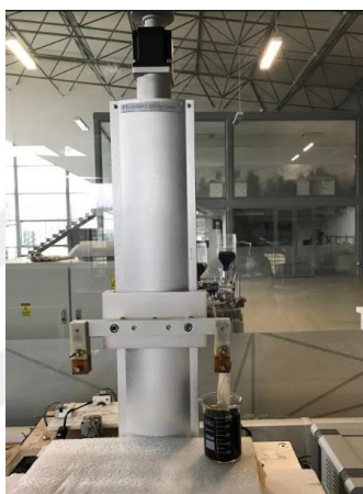
Figure 3.6: Dip-coating of PBI nanofiber produced at 15wt% using 50 mM catalysis concentration.
