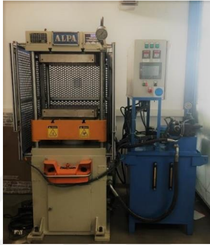
Figure 3.15: Hot press used for nanoprepreg production.
