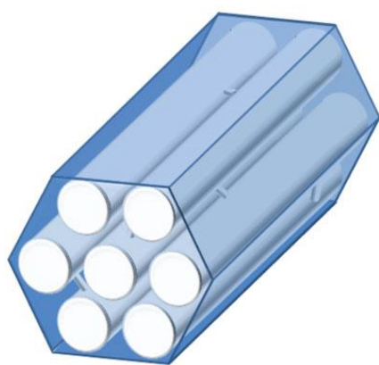
Figure 3: Representation of pore arrangement of ordered SBA-15 silica material [12]
