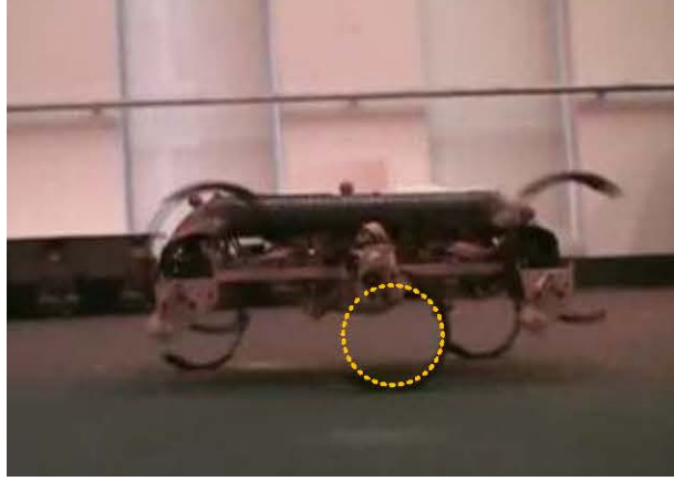
Figure 2.5: The confirmation of the circular leg assumption during dynamic running with a same leg used in this study.
