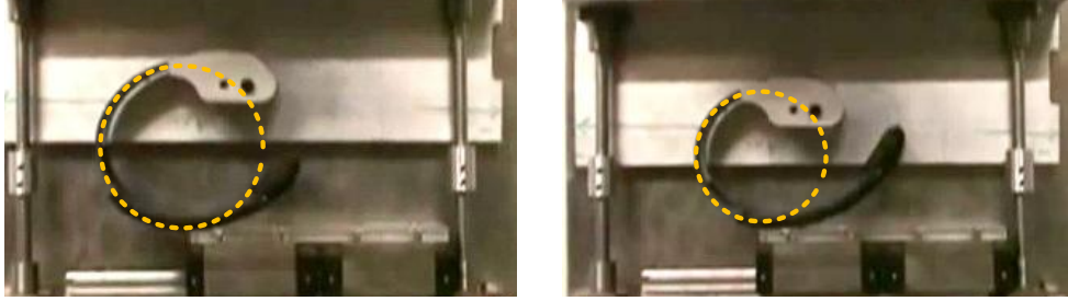
Figure 2.3: The images of a half circular leg in the experimental setup that is used to confirm our circular leg assumption for different compression levels. The leg properties are the same as that used in this study. We fit a circle to the deflected leg only considering the leg part between the hip and ground contact point.
