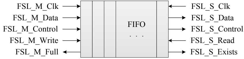
Figure 2.8: Block diagram of an FSL with Master and Slave signal interface.
