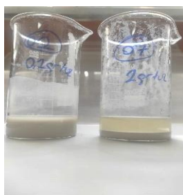
Figure 3.15: Salt-induced enhanced settling rate of the activated powder (Left is with 0.2 gr salt, Right is with 2 gr salt).
