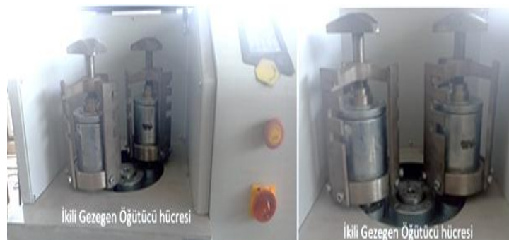
Figure 3.6: Planetary mill used in mechanical activation tests.
