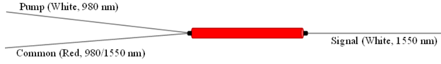
Figure 3.5. Basic scheme of WDM.
