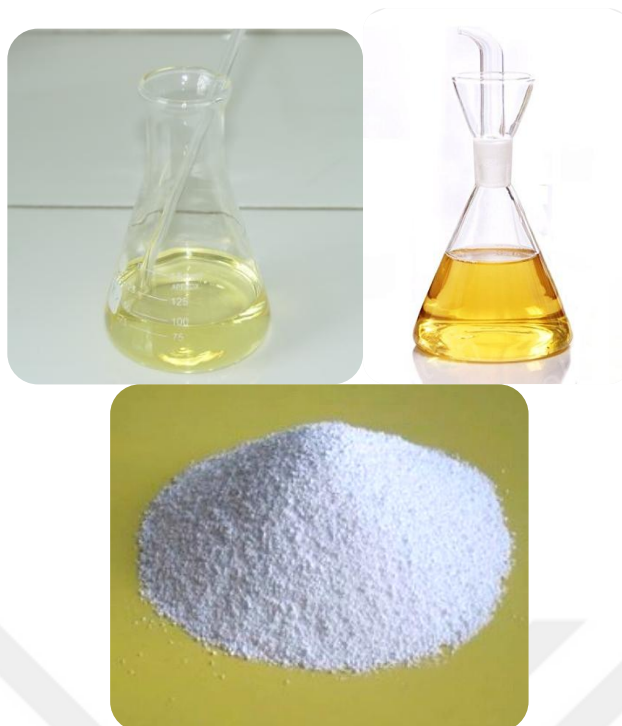
Figure 2.3: Chemicals used in dipping pretreatment; ethyl oleate, olive oil and potassium carbonate, left to right.
