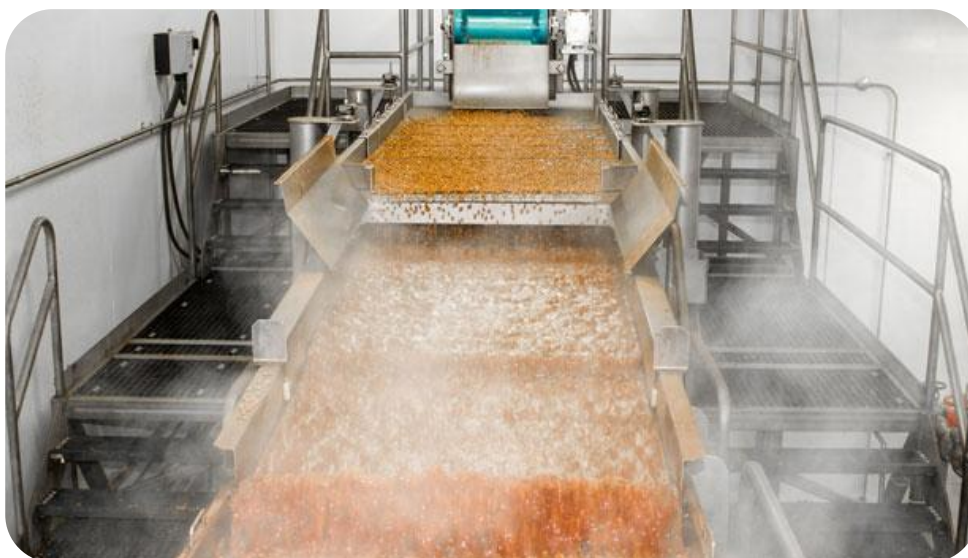
Figure 2.2: Industrial blanching application on almonds at Blue Diamond Growers, CA (Mikell Knights, 2014).
