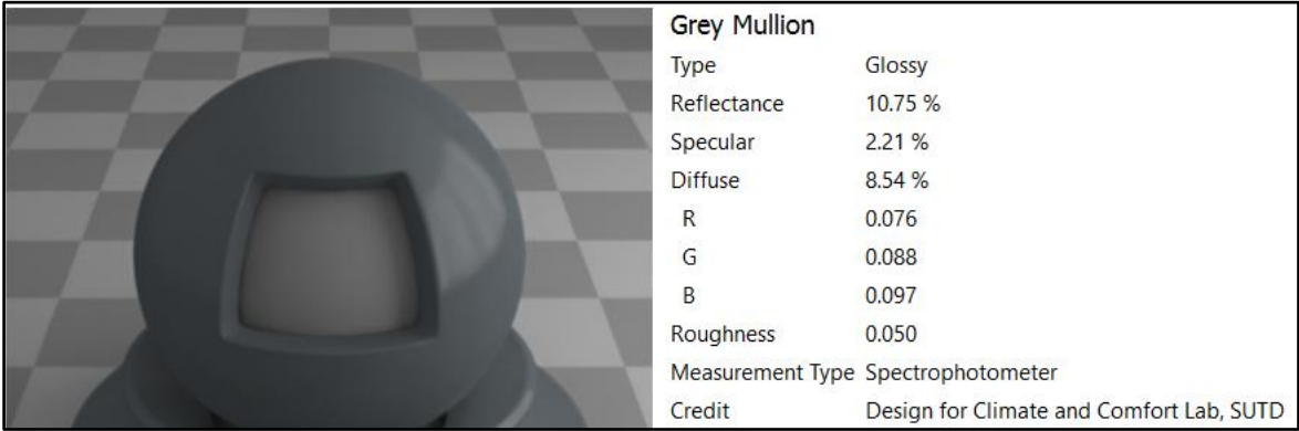
Figure 6.25. Mullion material detail.
