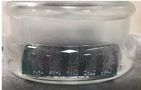
Figure 2.3: Wet Etching of micronozzle structures on the silicon wafer using KOH.
