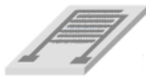
Figure 1.3 : Indium tin oxide glass microchip schematic diagram.
