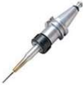
(b) Tool clamped to the holder extension with shrink fit
