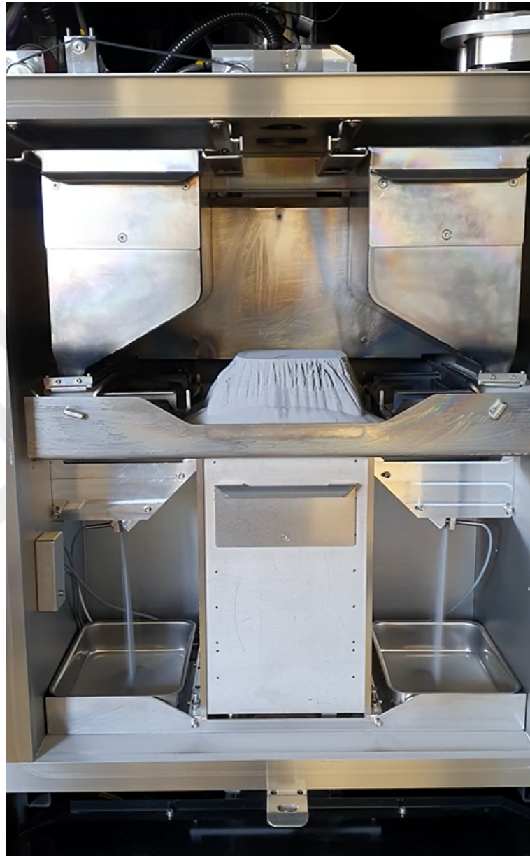
Figure 6.17: Block of powder containing the fabricated parts
