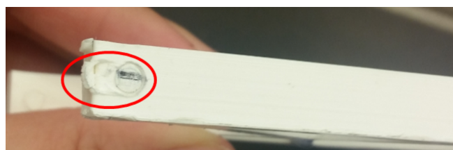
Figure 5.8: The trail of the screw on the cantilever beam part optimized by the SIMP method with a penalization factor of 3
