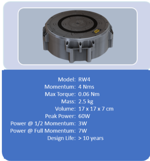
Figure 38: An example of reaction wheel as a suggestion for baseline design from Blue Canyon technologies [22]. A higher model with 8 N·m·s momentum is also available if necessarily.
