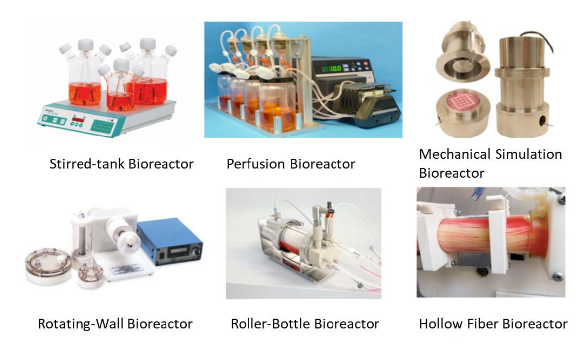
Figure 2.2. Different types of 3D cell culture bioreactors.
