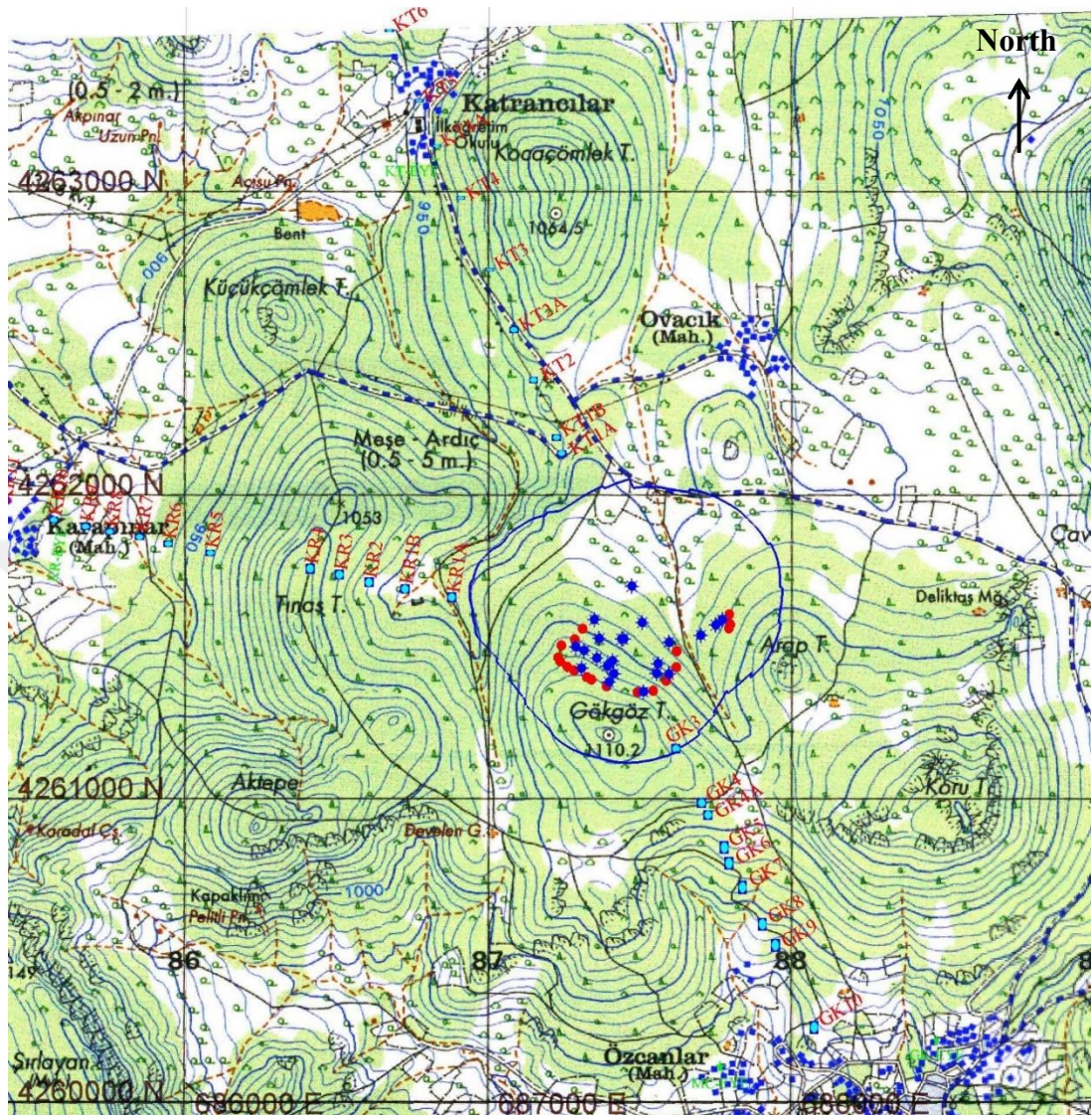
Figure 5.69 Topographic map Uşak Kışladağ Open Pit Mine with final outline of pit, neighboring settlements and monitoring paths (Çakmak, 2007)
