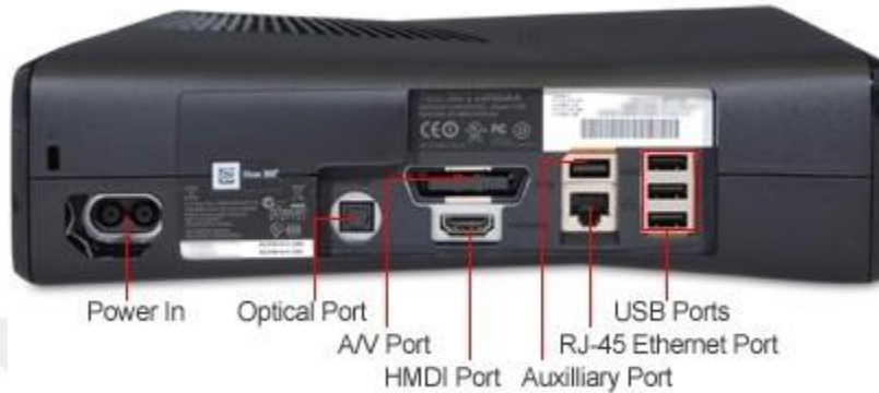
Figure 1.5 Xbox 360 Console Ports [17]
