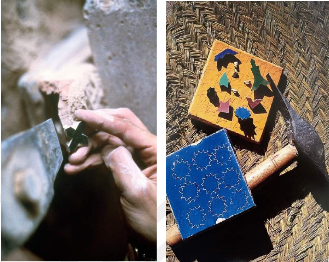
Figure 3.10 : Individual zellij pieces are cut from monochrome square tiles (Photos Left: Aga Khan Visual Archive (2017). Right: Castera (1999)).
