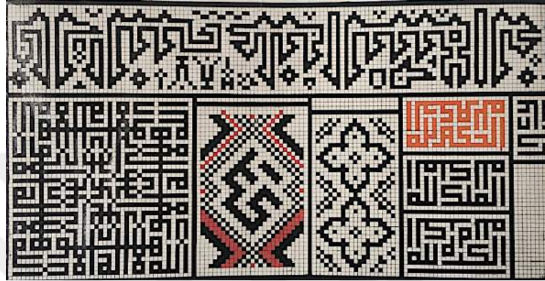
Figure 4.14 : Pattern number 51 from the Topkapı Scroll, a Naskhi inscription for Banna-i technique. Bricks fit to standard dimensions and scaling and the design matches a square grid (Necipoğlu, 1995, pp. 273 and 314).
