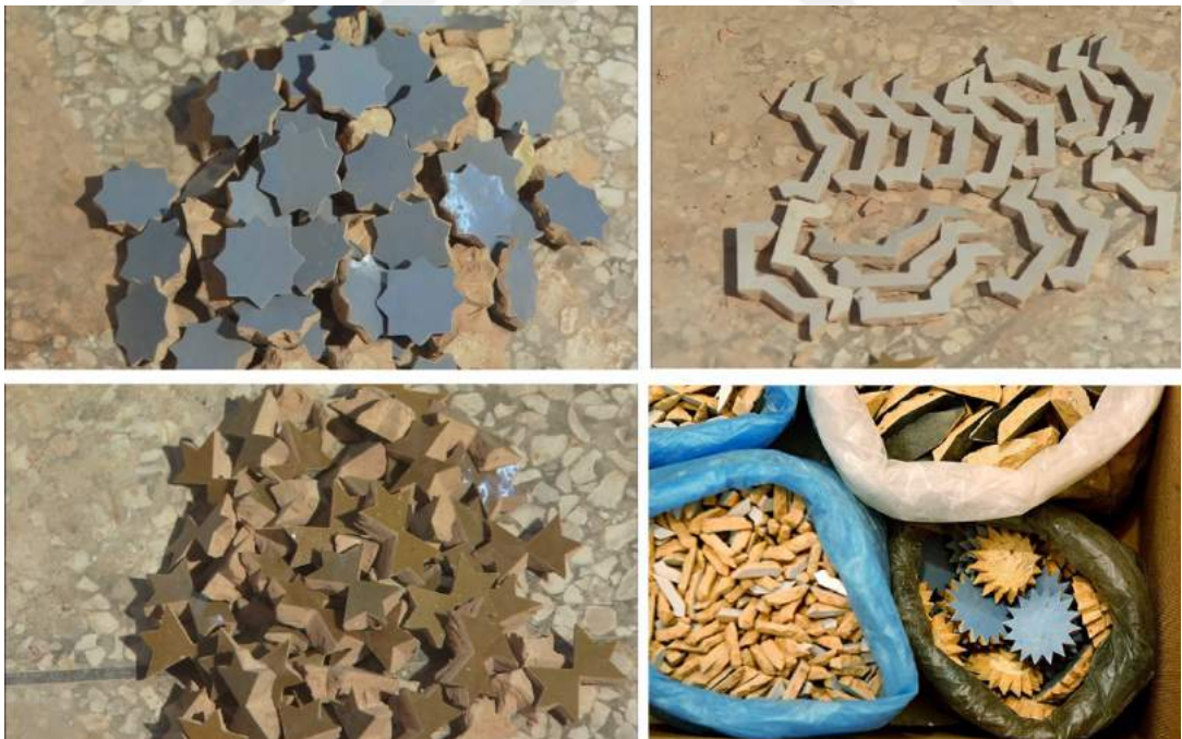
Figure 3.11 : The cutting results in a collection of individual zellij pieces, which are then filled into baskets or bags (Building the Moroccan Court, 2013).
