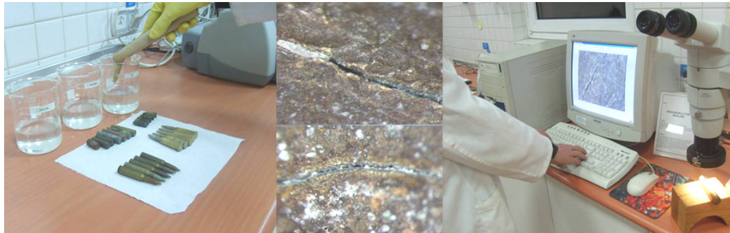
Figure 3.4.: Mercury Nitrate Test and Surface Examination Microscope in the physics laboratories.
