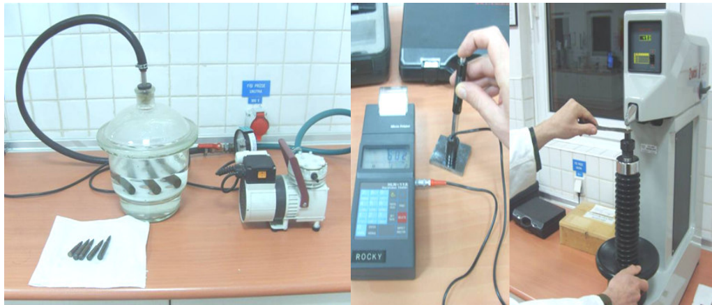
Figure 3.3.: Leak-proof and Metal Hardness Measurement Tests in the physics laboratories.
