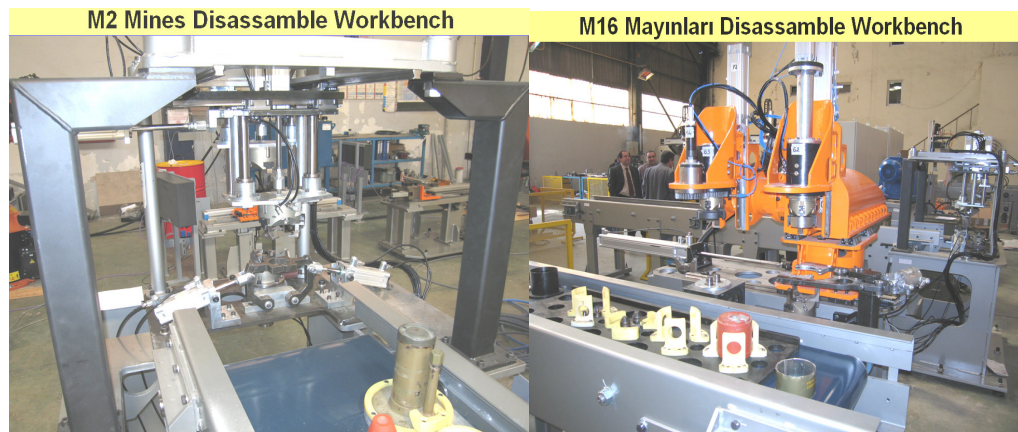
Figure 3.12.: Fuse Disassemble Units of Different Mines
