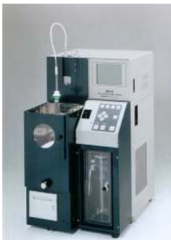
Figure 4.7. Tanaka AD-6 distillation analyzer
