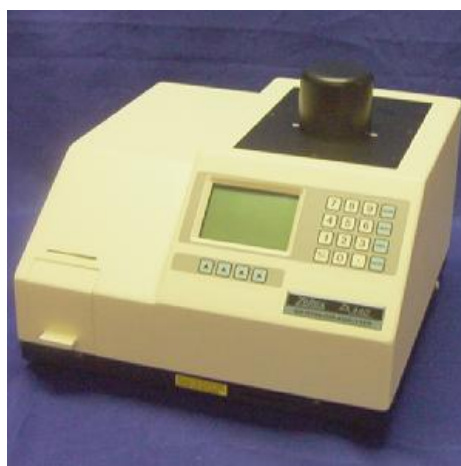
Figure 4.3. Octane Numbers Analyzer
