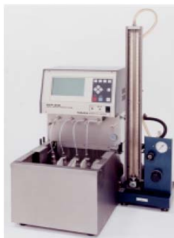
Figure 4.4. Reid Vapor Pressure (RVP) Analyzer
