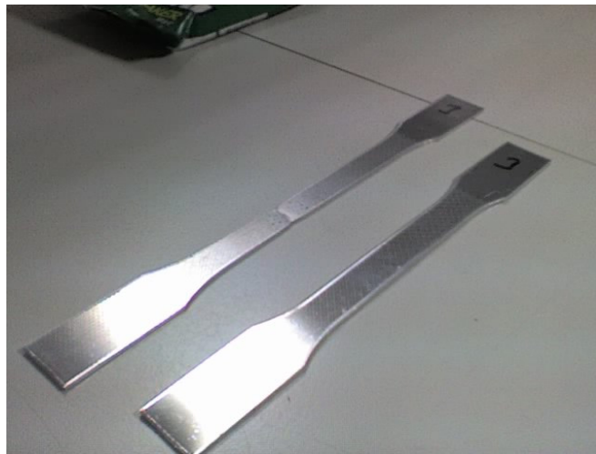
Figure 3.6. Electrochemically etched uniaxial tensile test specimens
