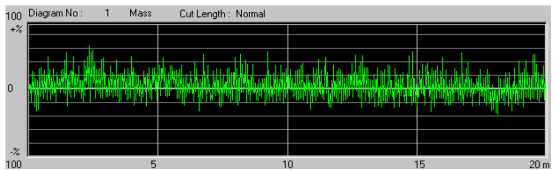
Figure 5.41. Mass diagram taken from Premier Tester 7000 of Ne 30-yarn
