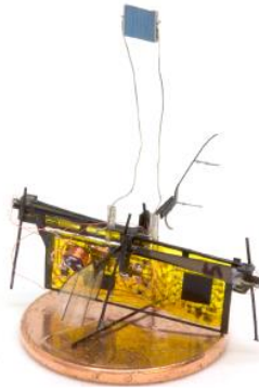
Figure 1.9 Full insect scale robotic fly placed on a US penny for scale [8].
