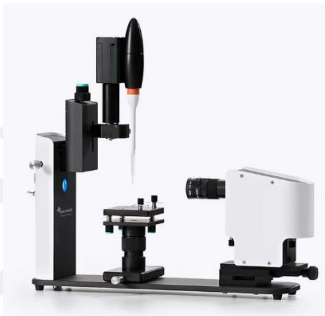
Figure 2.3: Contact angle measurement.
