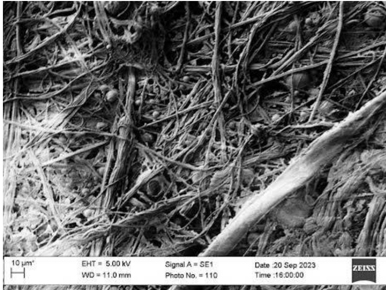
Figure 3.21: The sample formed when the substrate surface was first touched to the TMC organic solution
