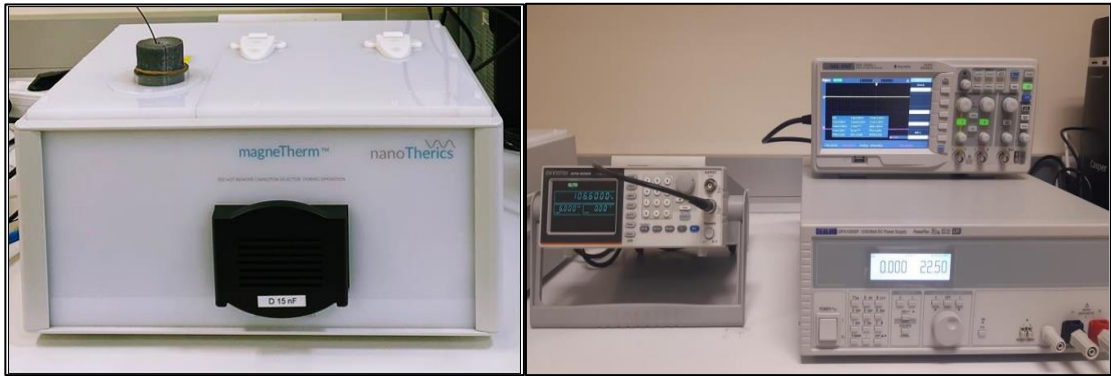
Figure 4.4. NanoTherics- MagneTherm Instrument (a), Control units that adjust the magnetic field amplitudes and frequencies (function generator, DC Power supply and oscilloscope)(b)
