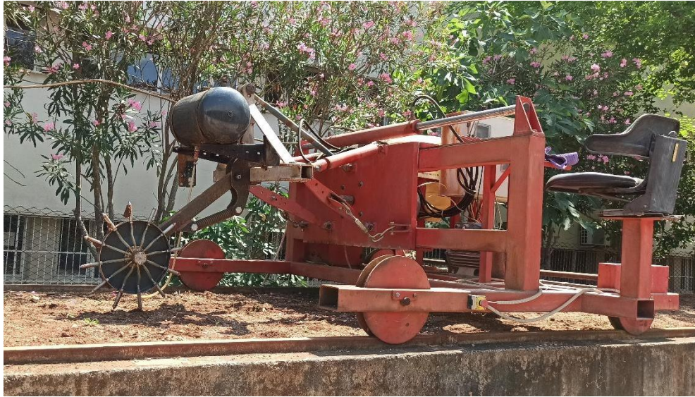
Figure 3.28. Installed Point Injection Liquid Manure system, little tank and air compressor on soil bin channel's moving carriage.
