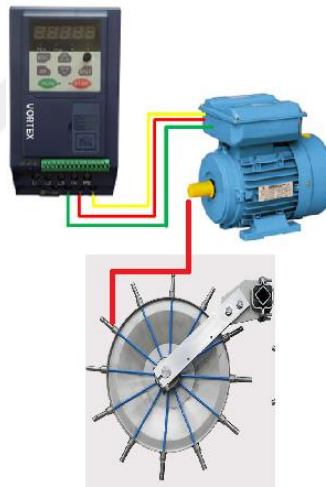
Figure 3.26. Forward speed simulated set.
