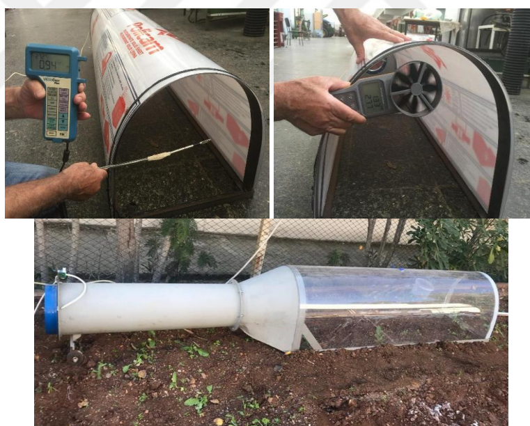
Figure 3.34. Installation the wind tunnel.
