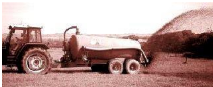
Figure 1. 1. Example of a broadcast spreader with a splash plate.
