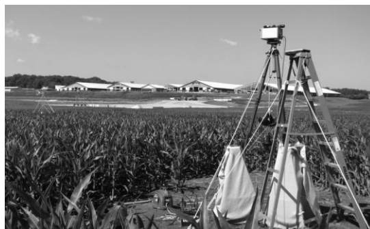
.Figure 1.7 Micrometeorology method for measuring whole - farm emissions.
