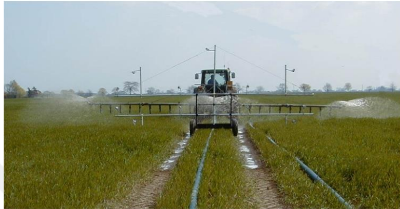
Figure 1.2. Example of apply liquid manure by irrigator.
