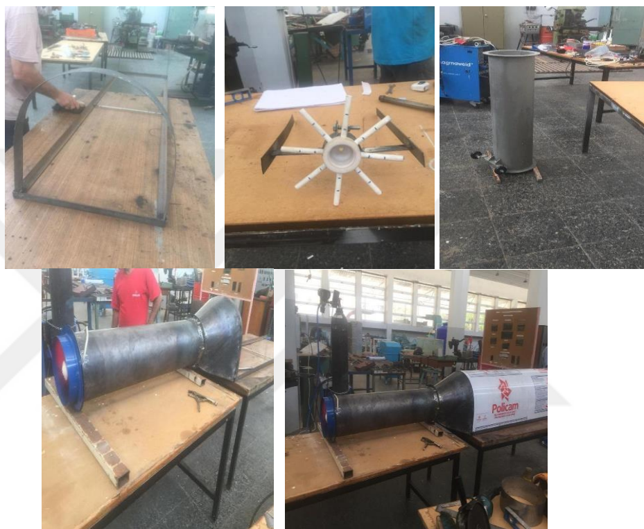
Figure 3.32. Wind tunnel manufacturing and assembly proses.
