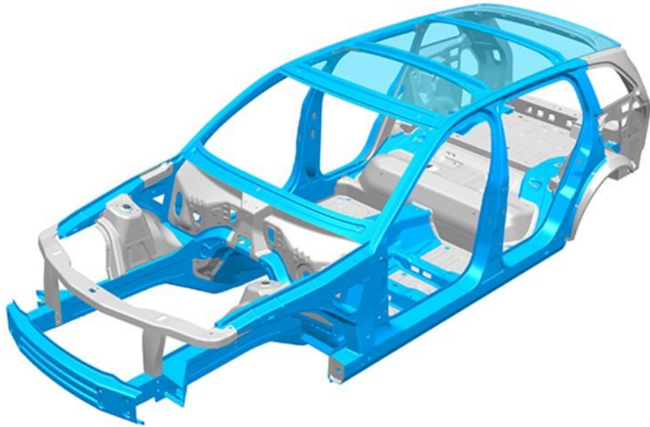
Figure 1-1 application of DP steel in a car body
