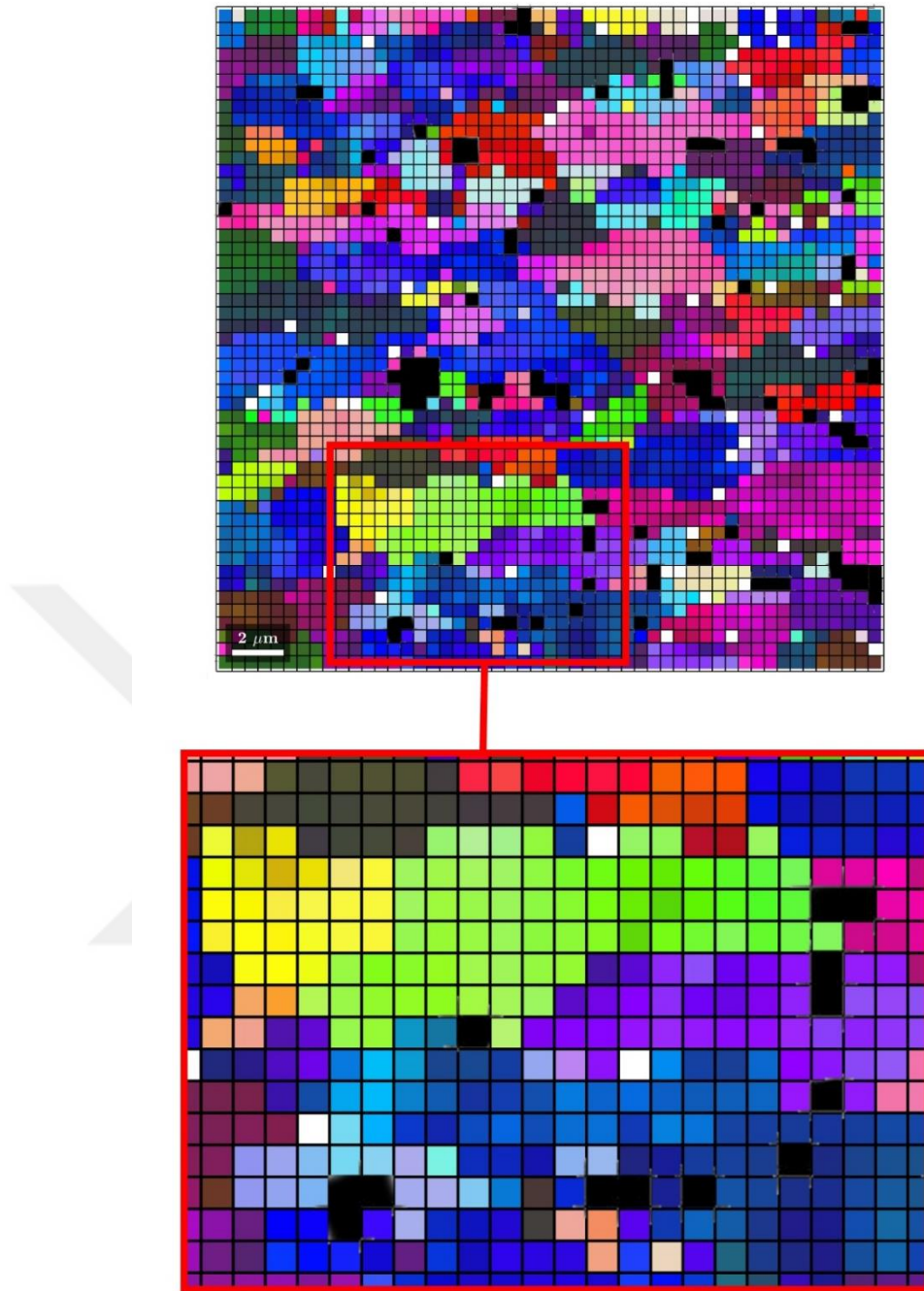
Figure 2-15 martensite grains superimposed on the grain distribution in 51x51 discretization plot, black squares represent martensite, areas with similar color tones represent a single grain of ferrite
