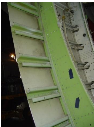
Figure 1.1 Metallic skin-stringer panel structure [1]
