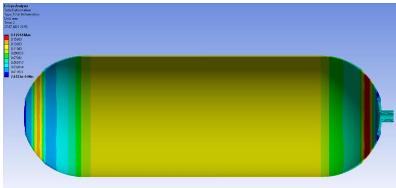
Figure 4.11 : Total deformation contour of spherical dome tank.
