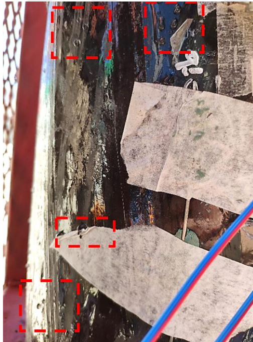
Figure 6.25 : Leakage of composite after LN2 test.
