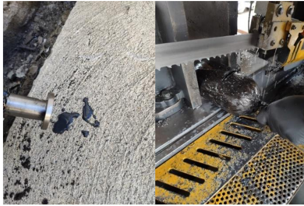
Figure 6.8 : Drain of acetone and composite tank cutting.
