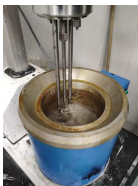
Figure 6.12 : Paraffin formulation preparation with melting pot and high shear.
