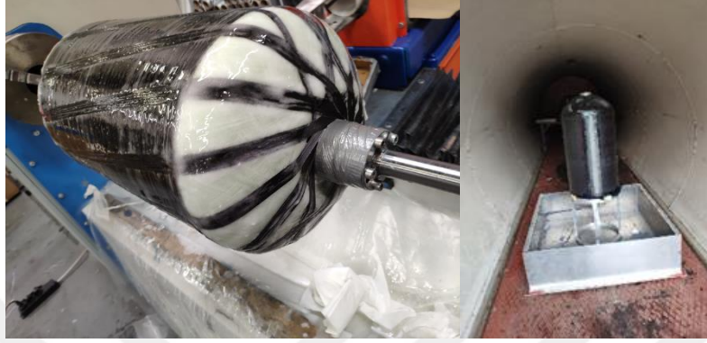
Figure 6.16 : Filament winding on paraffin mandrel and autoclave curing
