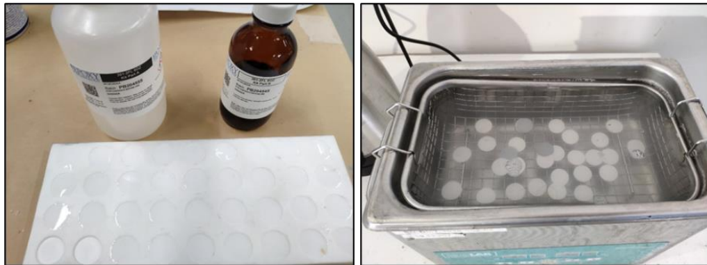
Figure 2.27 : LOX specimen mold and ultrasonic bath oxygen cleaning of specimens
