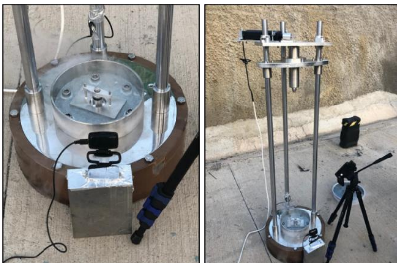
Figure 2.29 : LOX impact tests system and video recording.
