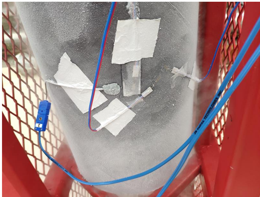
Figure 5.14 : Strain gagues on thermal cycle test
