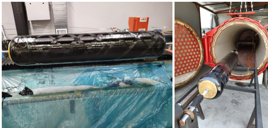
Figure 5.10 : Type-II composite vessel filament winding and autoclave process
