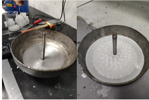
Figure 6.13 : Dome mold and liquid paraffin solidification
