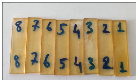
Figure 2.9 : Three-point bending tests specimens.
