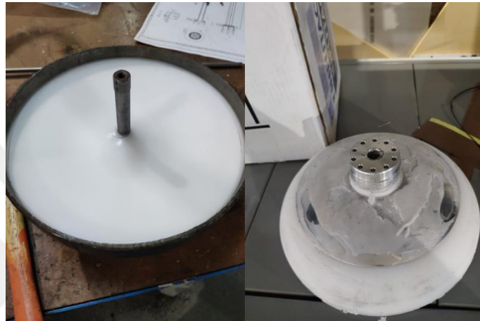
Figure 6.14 : Solid paraffin in mold and released paraffin dome with metal boss.
