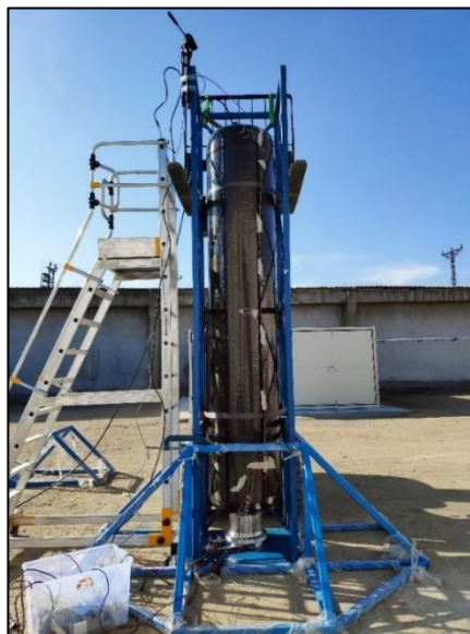
Figure 6.31 : Hydrotest system of Type-V pressure vessel.
