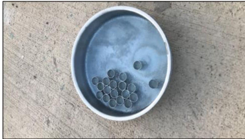
Figure 2.28 : Oxygen soaking of epoxy samples in cups before test
