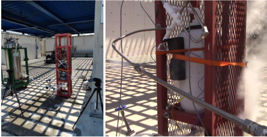
Figure 6.22 : (a) Cryogenic testing setup, (b) Cryogenic Filling.
