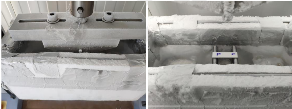
Figure 2.13 : LN2 submerged three-point bending test of Epotek T7110 epoxy system.
