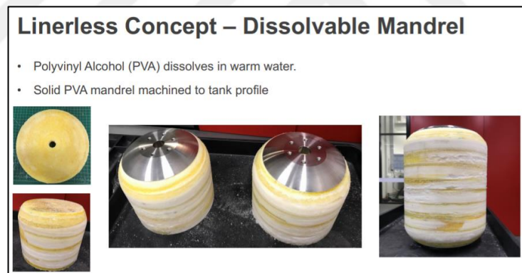
Figure 6.2 : Dissolvable mandrel with PVA material [116].
