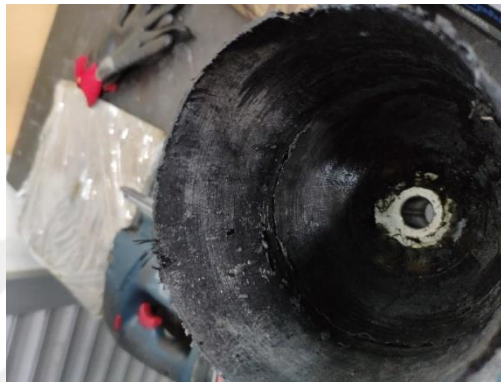
Figure 6.9 : Half cut section of the winded vessel.
