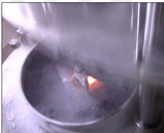
Figure 2.30 : The explosion moment of Epotek 301-2FL epoxy system.
