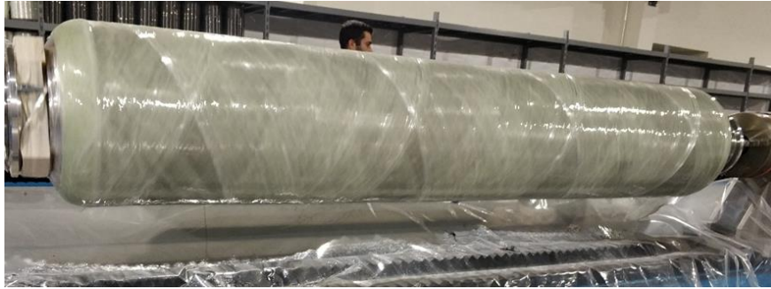
Figure 6.29 : Glass Layer Winding.
