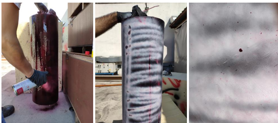
Figure 5.12 : NDT check for detecting manufacturing based cracks
