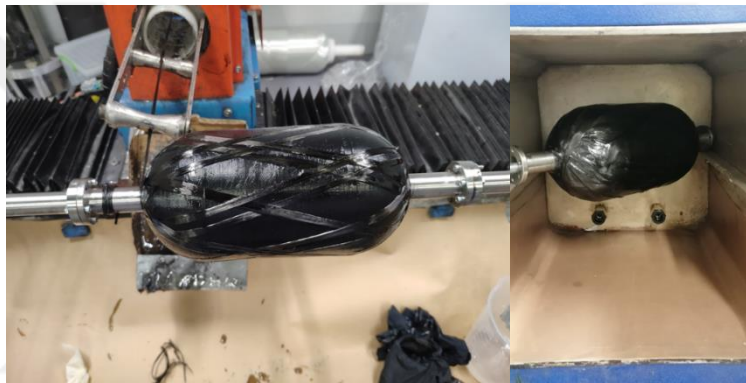
Figure 6.7 : 3D printed mandrel filament winding and oven curing.
