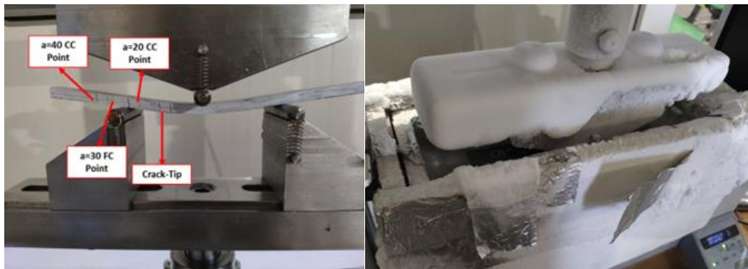
Figure 3.6 : ENF test performed in (a) RT environment; (b) LN2 environment.
