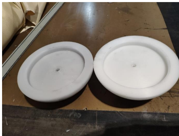
Figure 6.15 : Dimensionally refined paraffin domes.
