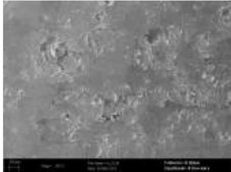
(c) 4 bar, 100mm SoD, 3 seconds - magnification 200X
