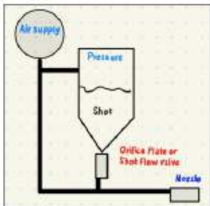
(c) Direct pressure delivery system
