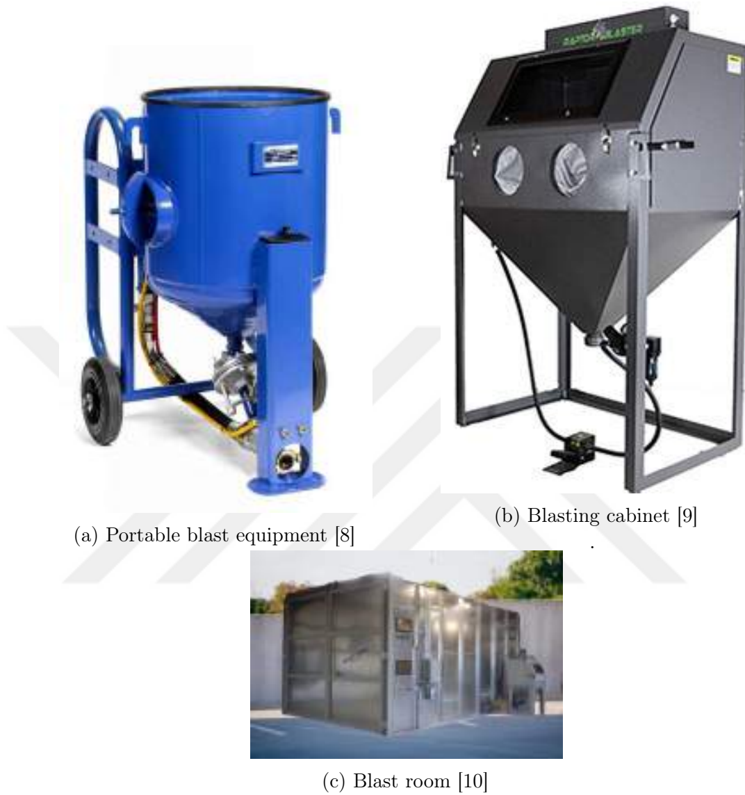
Figure 1.2: Blasting machine types
