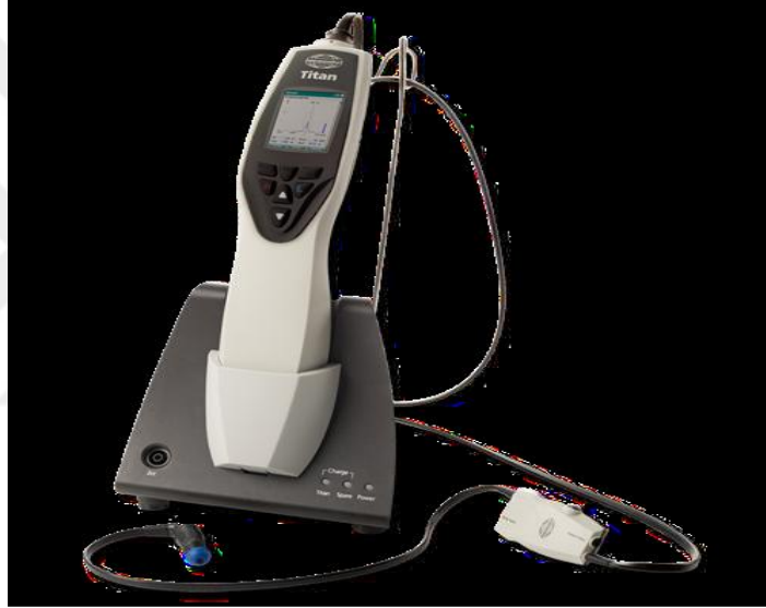
Resim 1. Interacoustics Titan Geniş Bant Timpanometre ( Hunter ve Shahnaz, 2014)
