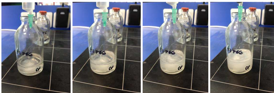
Figure 4.2. Spontaneous formation of nanocapsules with nanoprecipitation
