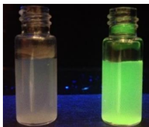
Figure 3.15. Photograph of UV-illuminated aqueous solutions of NG2 after treated with BODIPY-Br (Left) BODIPY-SH (Right)
