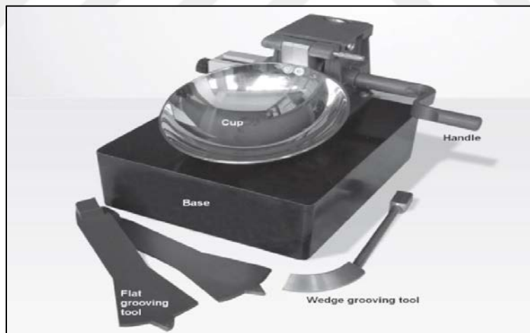
Figure 2.1 the Casagrande's apparatus. [2]
