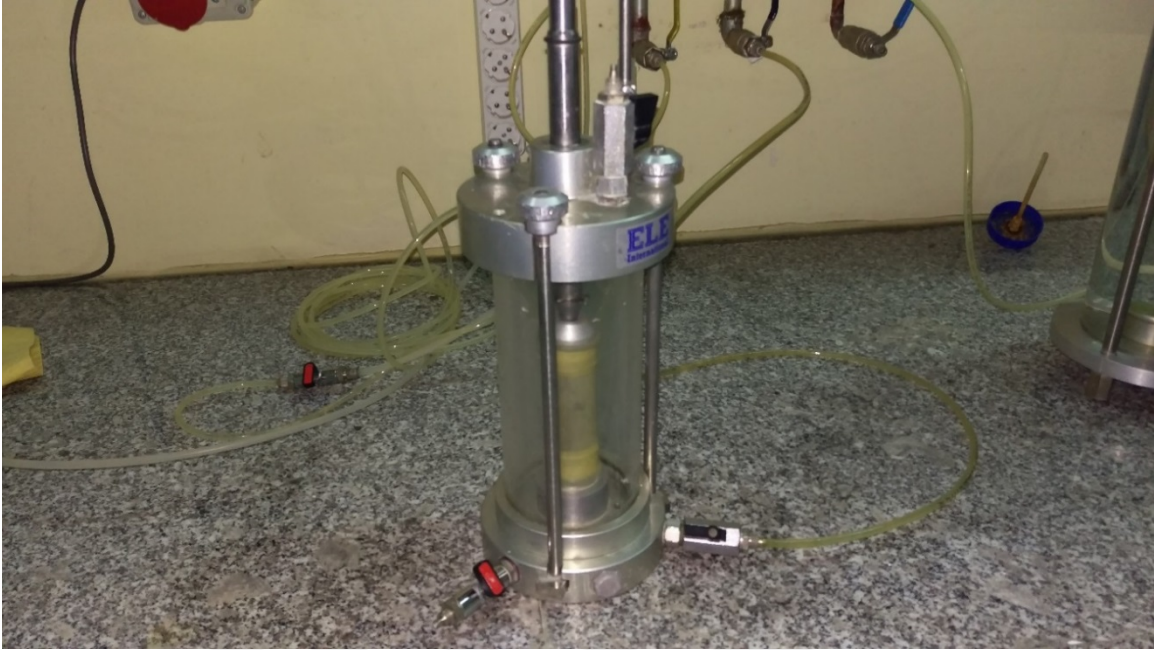
Figure 3.19 The cell is filled with the water
