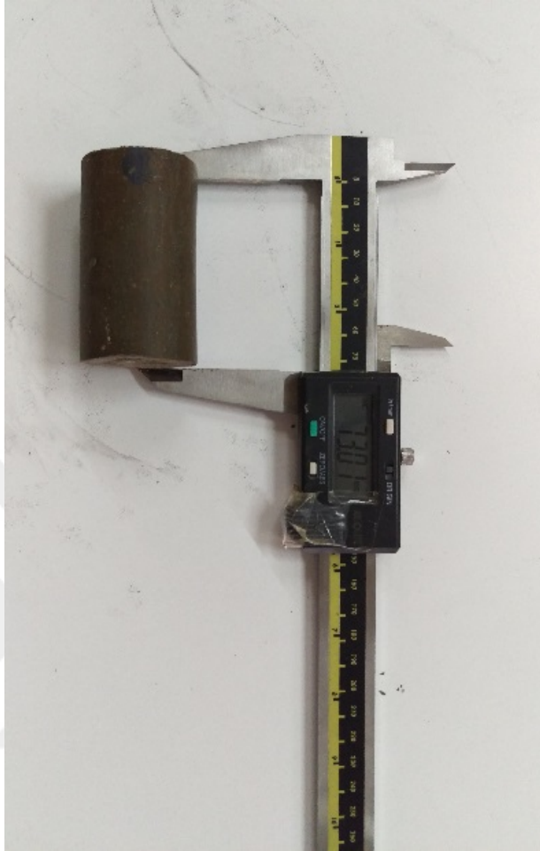
Figure 3.15 The picture shows measuring the height of the sample Then, samples were placed in the device between two plates to make sure that the pressure is equally distributed as shown in figure
