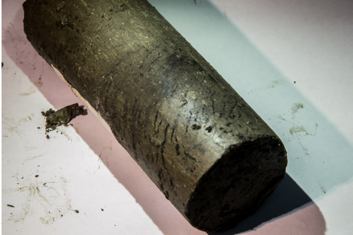
Figure 4.21 the decay on the surface of the soil sample due to storage for 90 days
