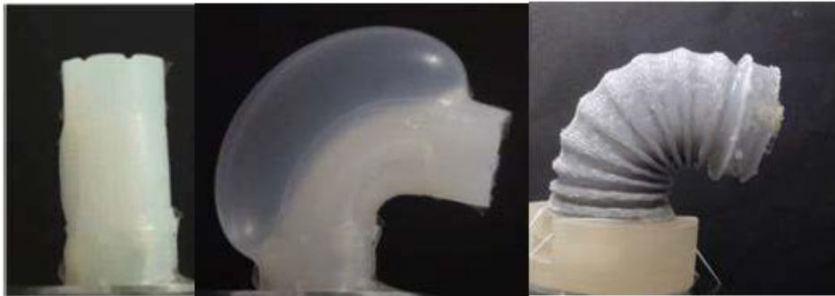
Figure 2.8. One of the air chambers of the STIFF-FLOP manipulator is inflated.
