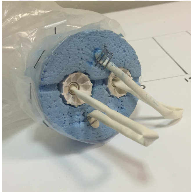
Figure 4.3. Tip of the robot made of styrofoam when the slack section remains out of the robot.
