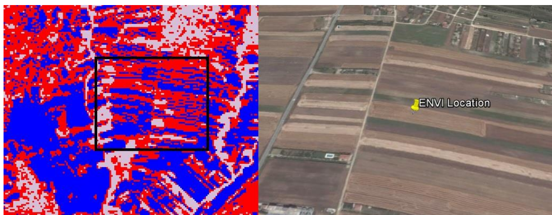
Figure 5.12 : Missclassification of bare land as impervious surface in NDBI image Landsat5 TM August 20, 2003 in contrast to Quickbird August 03, 2003 image.
