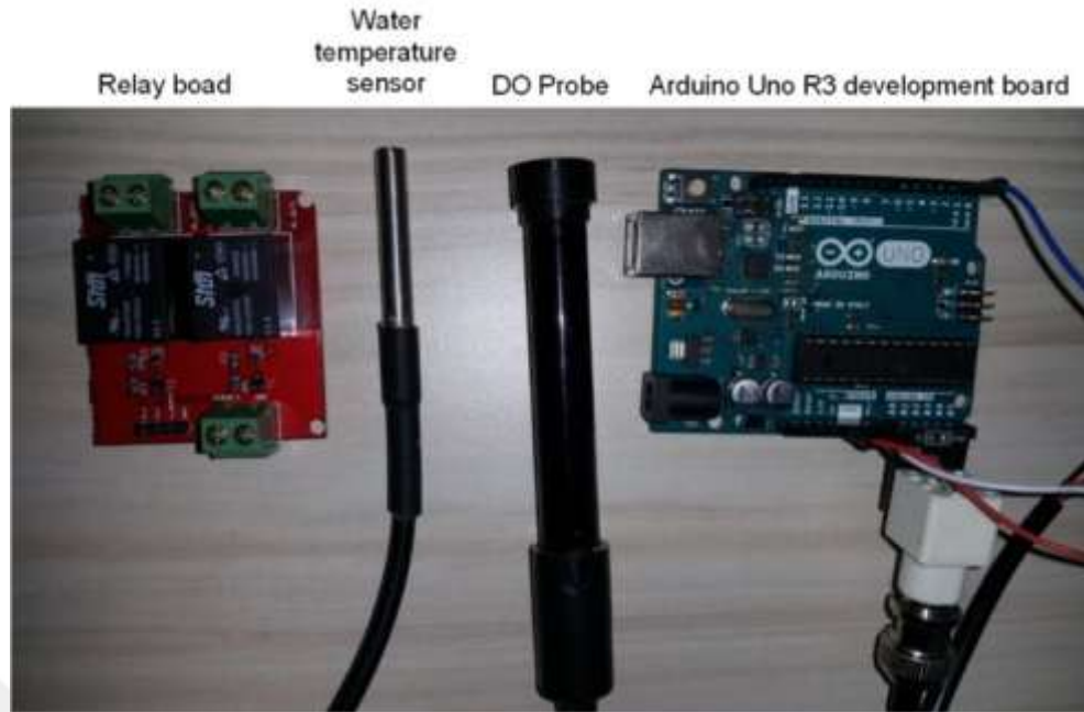
Figure 5.10 Aeration system control unit
