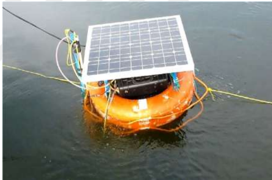
Figure 3.5 Solar driven floating type aerator (Solpico et al. 2014)
