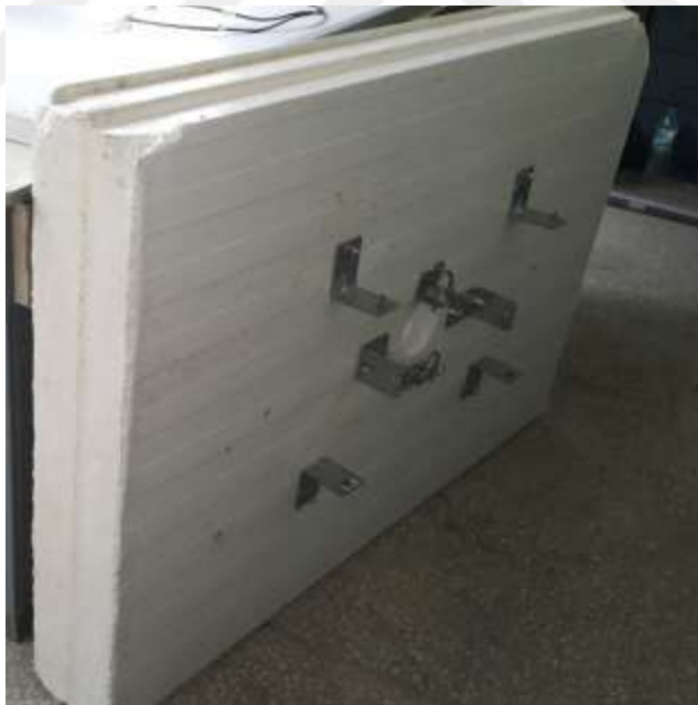
Figure 5.8 Floating platform constructed for Prototype II
