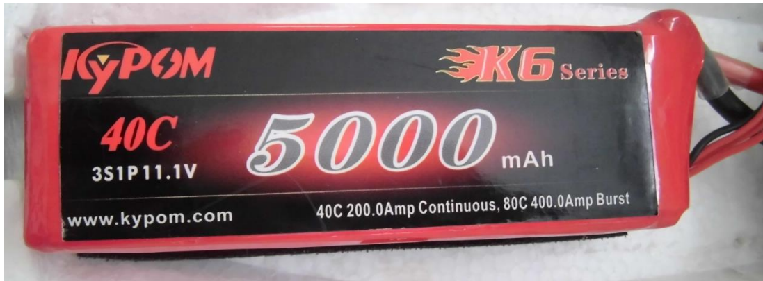
Resim 3.5 KyPOM 3s 5000mah 40c lipo batarya.
