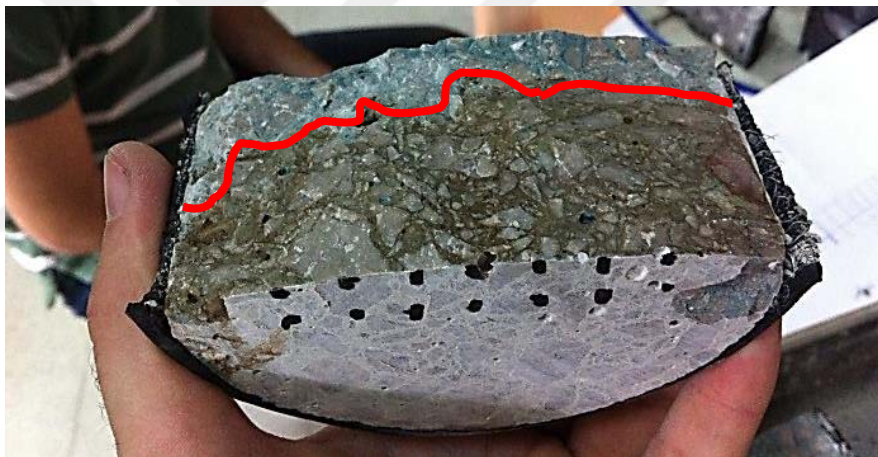
Figure 3.12 Half slice of specimen after completion of the test and red line shows penetration depth of chloride-ions
