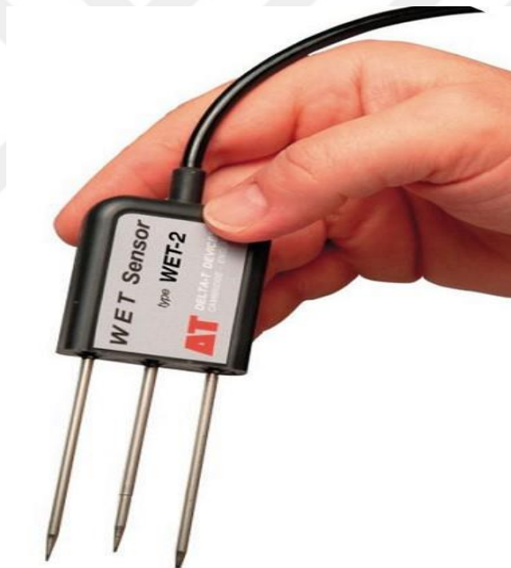
Figure 2.10: Soil salinity sensor (Url-5).
