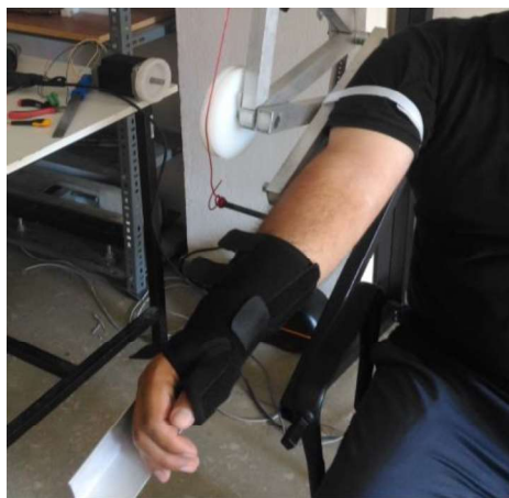
Figure 50. Attachment of the Human Arm to the System
