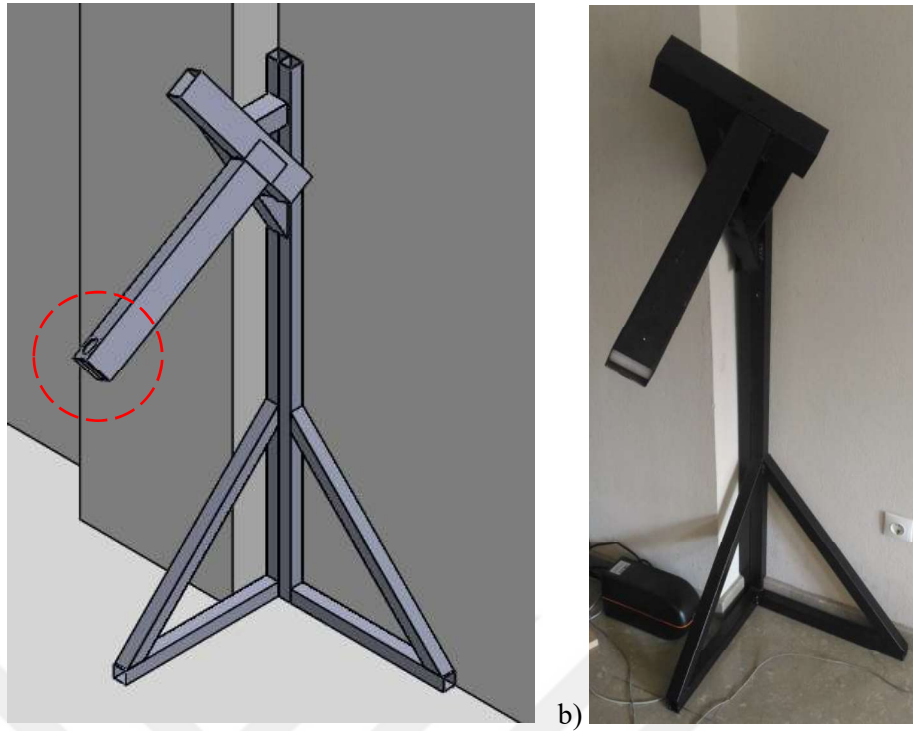
Figure 40. The Base Design: a) the CAD Model and b) the Manufactured Base
