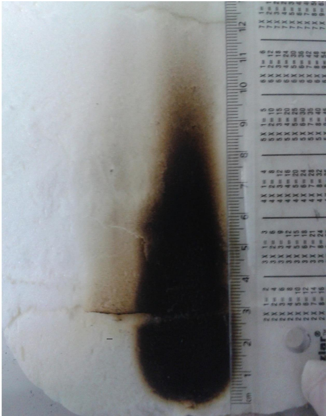
Figure A.9 : TCPP (20 % in polymix) at polyurethane rigid foam (9 cm)
