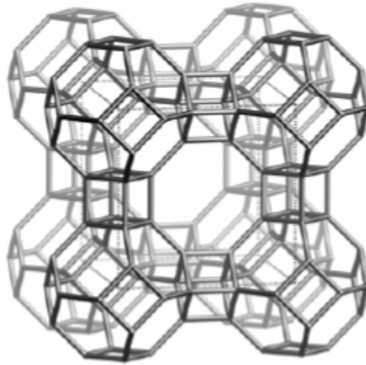
Figure 2. 6. Framework of Zeolite A [Database of Zeolite Structures]
