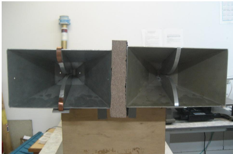
Figure 5.3 The double ridge horn antennas used in the measurement setup (left hand side antenna is the transmitting antenna; right hand side antenna is the receiving antenna).
