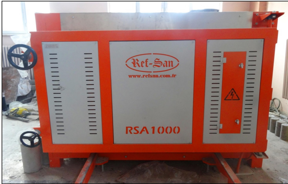
Figure 3.12 The furnace used to curing of SCGC specimens
