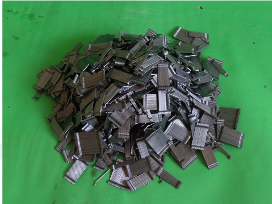
Figure 3.3 Hooked-end steel fiber used in SCGC
