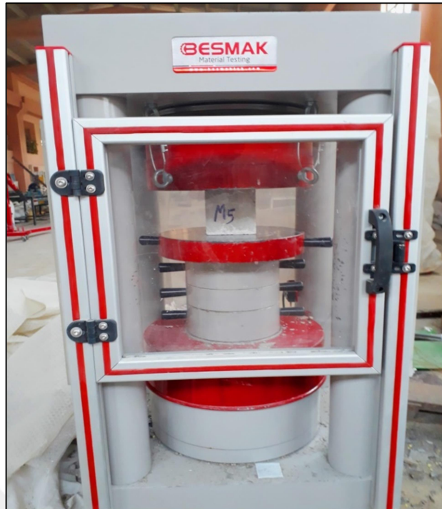
Figure 3.13 A specimen under compressive strength machine
