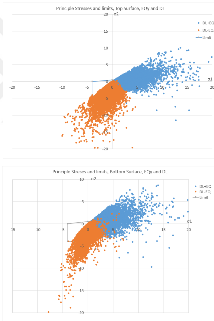
Figure 3.34. Limits of principle stresses using Coulomb-Mohr Theory
