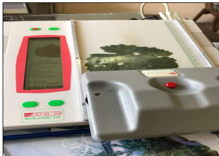
Figure 3.7. Leaf area meter AM-300, 2003ADC, UK
