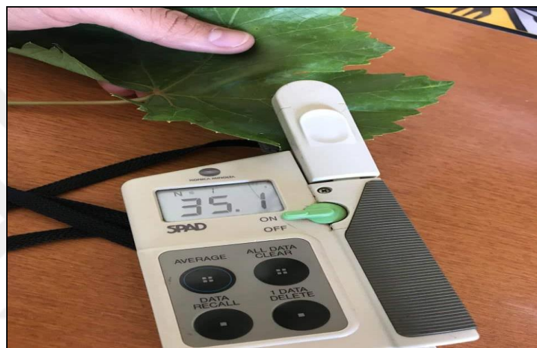
Figure 3.8. Estimation of leaves chlorophyll using SPAD-502-meter, Japan.
