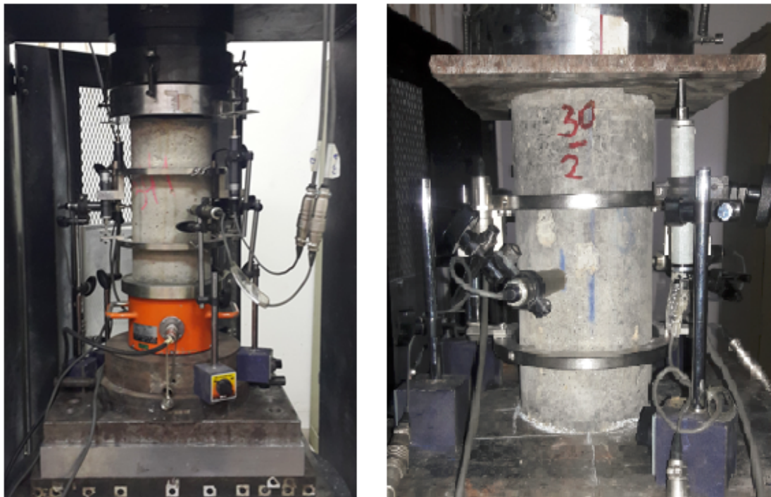
Figure 4.47: Typical cylindrical specimens for Poisson's ratio test.
