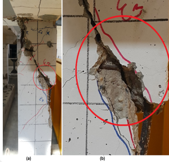
Figure 4.46: (a) Failure mode of the specimen RCF-2 at the end of the test, (b) stirrups failure due to corrosion
