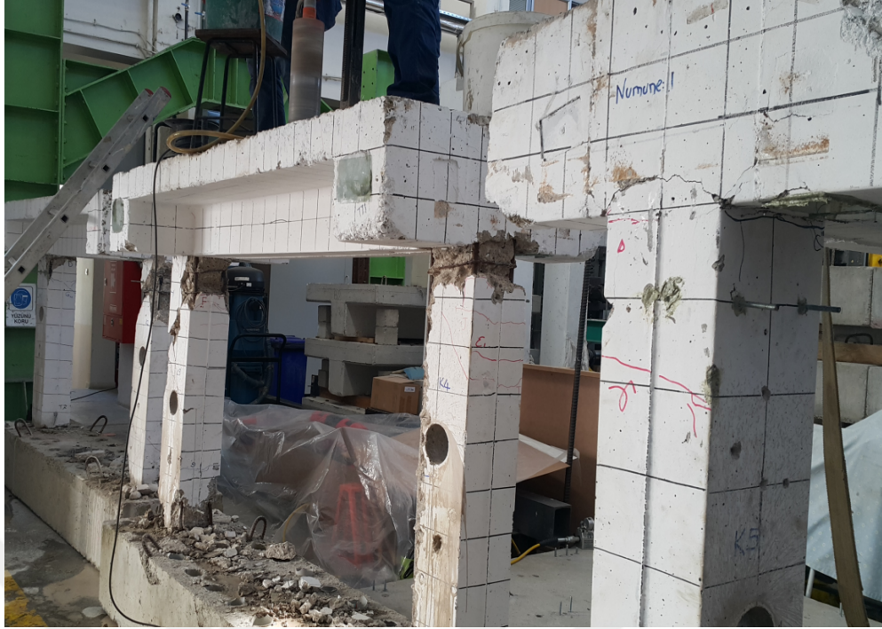
Figure 4.19: Taken of core specimens from tested RC frame with core holes.
