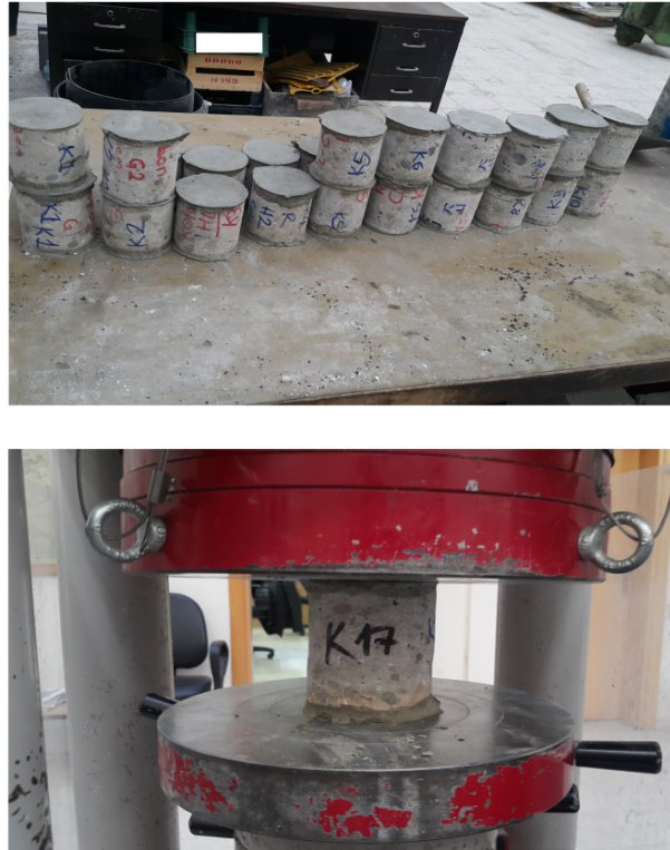
Figure 4.20: Core specimens and testing equipment of press tool.
