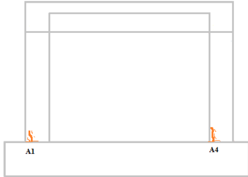
Figure 4.34: Crack pattern of RCF-2 before the experiment
