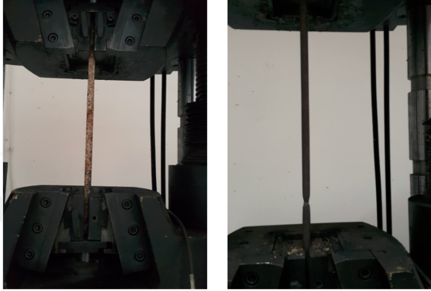
Figure 4.23: Tensile test of corroded reinforcement bars.
