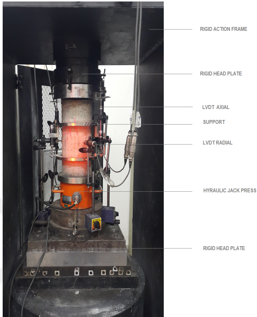
Figure 4.49: Testing instrument of the Poisson's ratio measurements.
