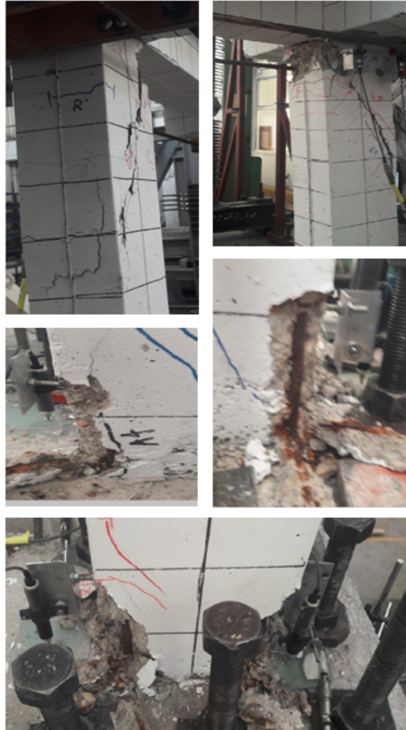
Figure 4.45: Demolished part of the specimen RCF-2 at the end of the test
