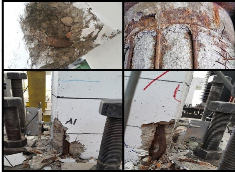
Figure 2.1: Natural corrosion process and cover concrete cracking.
