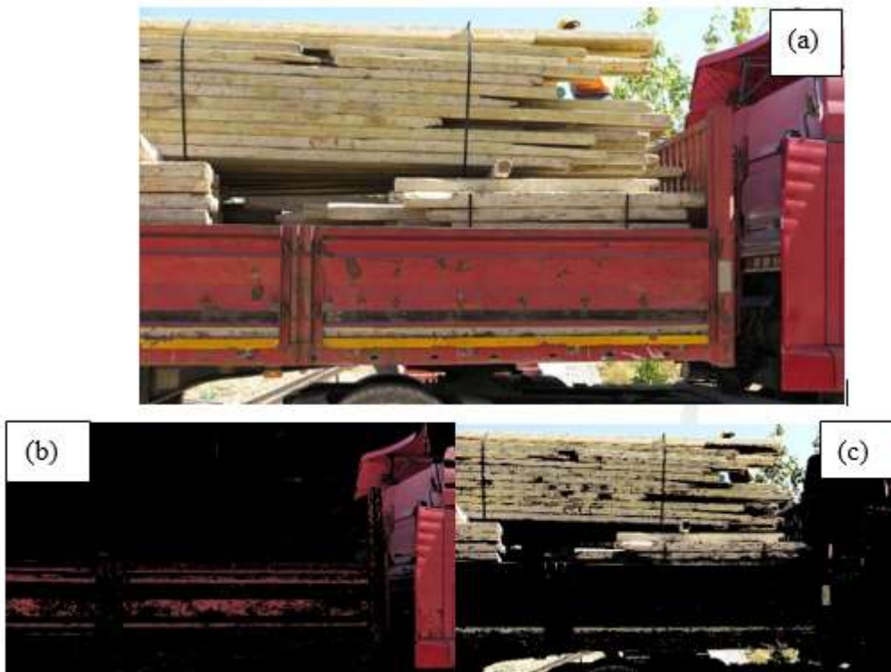
Figure 120 Loaded truck image with extracted (b) Truck (c) Loaded Formwork.
