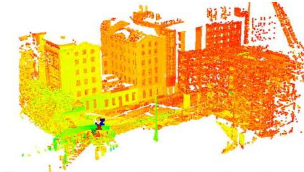
Figure 6 A point cloud containing millions of points of an under construction structure [48].
