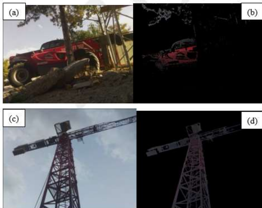
Figure 119 (a)-(b) Boom loader detected (c)-(d) crane detected by K-means clustering in SCAER.
