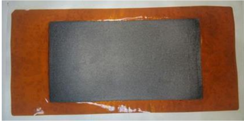
Figure 3.5. HT-PEMFC MEA (acid-leaching PBI membrane and GDE)
